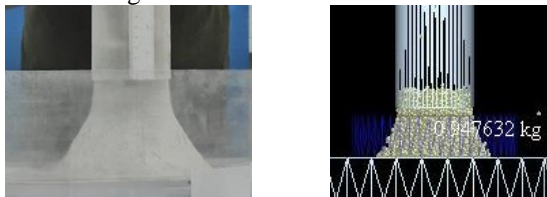
Fig. 5 Static angle of repose – model calibration (motion capture), left – real test, right - simulation
