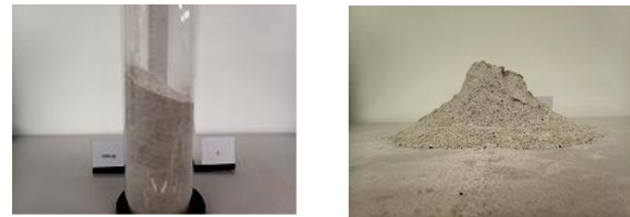
Fig. 1 Static angle of repose – pipe test
