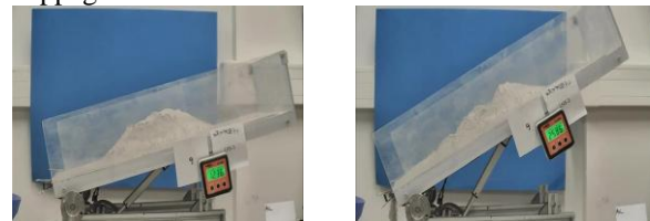
Fig. 3 External friction angle/equipment interaction – platform test
